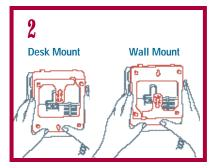
Attach the wedge-shaped base in desk mount or wall mount† position.
