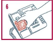
Attach the receiver card and lens (shiny-side down).
